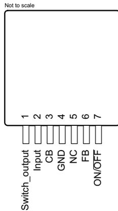
Figure 5-1. KTW Package 7-Pin TO-263 Top View
