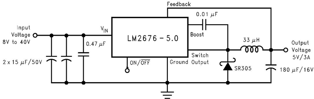
Figure 8-1. Basic Circuit for All Output Voltage Versions
