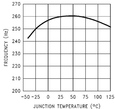
Figure 6-10. Switching Frequency
