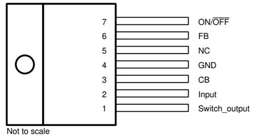
Figure 5-2. NDZ Package 7-Pin TO-220 Top View
