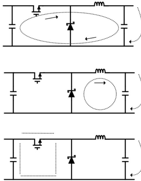
Figure 8-8. Typical Current Flow on a Buck Converter
