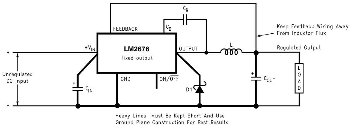
**Figure 8-6. Basic Circuit for Fixed Output Voltage Applications.**
