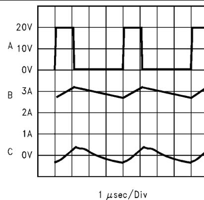
Continuous Mode Switching Waveforms  $V_{IN} = 20\text{ V}$ ,  $V_{OUT} = 5\text{ V}$ ,  $I_{LOAD} = 3\text{ A}$   $L = 33\text{ }\mu\text{H}$ ,  $C_{OUT} = 200\text{ }\mu\text{F}$ ,  $C_{OUTESR} = 26\text{ m}\Omega$
